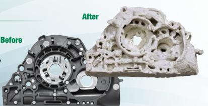
Automotive parts made from LGF Compounds showing before and after resin burn off, which exposes the LGF skeleton structure.
