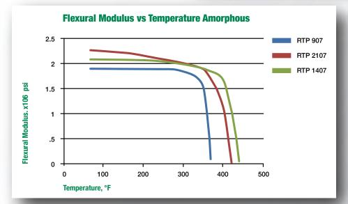
Note that the amorphous polymers have a moderate and steady loss of properties until they approach their Tg. Then they rapidly lose strength and stiffness and become incapable of carrying a load.
