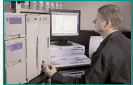
Nanotubes allow compounds to meet the stricter cleanliness requirements of the electronics industry. Shown here is an RTP Company R&D engineer using a gas chromatograph to test a nanotube compound for ionic contamination.
