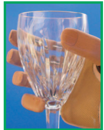
Prosthetic fingers overmolded with TPE
