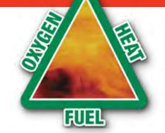
The goal of flame retardant technology is to disrupt one or more of the fire triangle elements necessary for combustion
