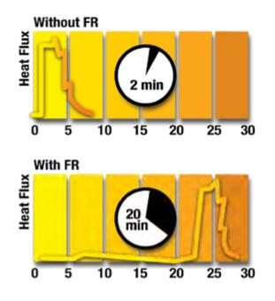
Burning behavior of plastics is not just a material characteristic. Part design and nominal wall thickness are key factors in flammability certification.
