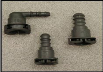
Fuel line components PPA, Nylon, Acetal
