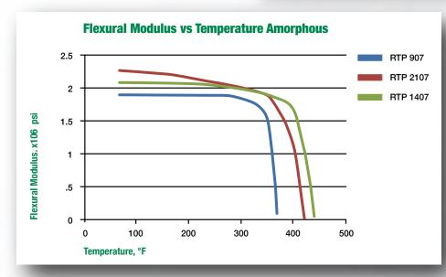
Note that the amorphous polymers have a moderate and steady loss of properties until they approach their Tg. Then they rapidly lose strength and stiffness and become incapable of carrying a load.
