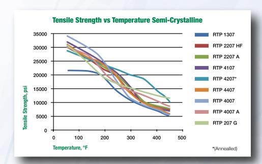
Note that all the semi-crystalline polymers start with fairly high properties that gradually decline. As they near the Tg, the slope of the reduction increases. Then, unlike amorphous polymers, the rate of loss stabilizes and they remain useful until they get near their melting point.
