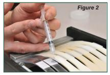
The test procedure consisted of molded ASTM D638 Type 1 tensile bars, which were placed in a specially designed fixture to ensure the samples were strained to 1.0% (Figure 1). A gauze patch was applied to the center of the specimen and saturated every 24 hours with a specific chemical agent (Figure 2). This allowed the material to air dry and oxidize as would be seen in a typical field exposure. The testing was performed on each composition in triplicate to confirm consistency.
